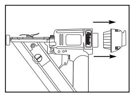
Figure 7. Removing nailer exhaust cap.
